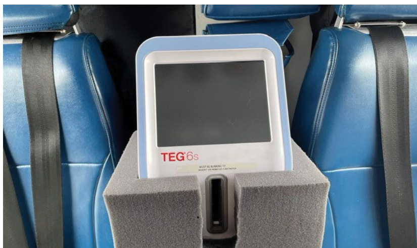
Secured in the back of the Base 6 aircraft, this TEG machine tests blood samples to determine its clotting capacity.
