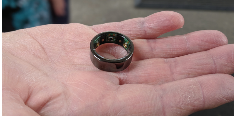
The Ora Ring tracker monitors an individual’s body temperature, breathing, heart rate and other vital signs.
